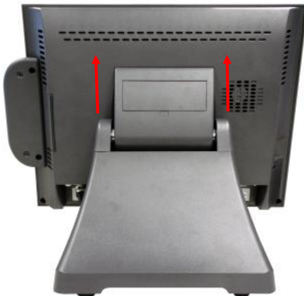
b. Lift the panel up and separate it from the stand bracket
