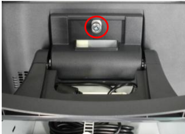
a. Loosen the thumbscrew (1)
